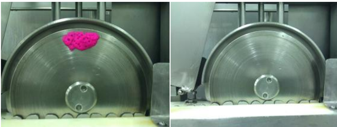
Figure 4. TBF 300 foam applied on a slicer that is frequently cleaned and disinfected by hand. No biofilms were detected. This result is consistent with low values of ATP luminescence detected and absence of microbiological contamination.
