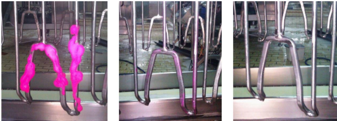
Figure 1. TBF 300 was applied on a poultry hanger after cleaning and disinfection (left). After rinsing, residual coloration was observed, indicating presence of biofilms (centre). The hanger was subsequently cleaned and disinfected using biofilm-removal detergents and the TBF 300 test was performed again. After rinsing, surfaces were clear of dye, indicating the biofilms were removed (right).
