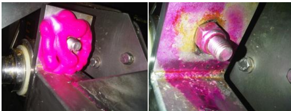
Figure 2. TBF 300 foam applied on a hard to reach spot for cleaning operations. After rinsing a strong presence of biofilms is detected.
